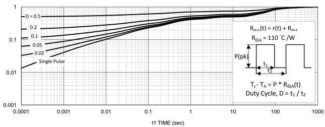
11. Normalized Thermal Transient Junction to Ambient
