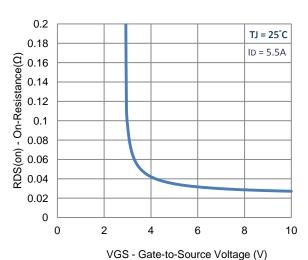
3. On-Resistance vs. Gate-to-Source Voltage
