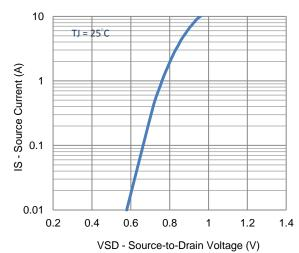
4. Drain-to-Source Forward Voltage
